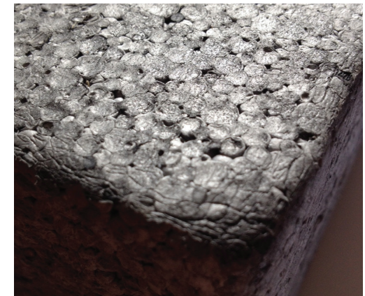
Examples of moisture-open (wood fibre board) and moisture-closed (EPS) insulation materials
